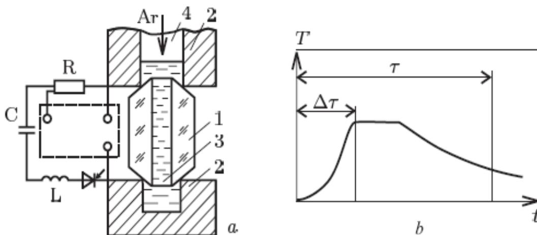
Figure 2. Schematic diagram of setup for isobaric heating in a transparent capillary. (a): 1 - capillary; 2 - electrodes; 3 - liquid cesium; 4 - argon purge. (b) The behavior of the time dependence of plasma temperature.
