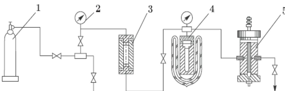
Figure 1. The schematic diagram of experimental facility for the generation and investigation of nonideal plasma of metals. 1 - cylinder with argon; 2 - pressure gauges; 3 - argon cleaning system; 4 - thermocompressor; 5 - high-pressure chamber.
