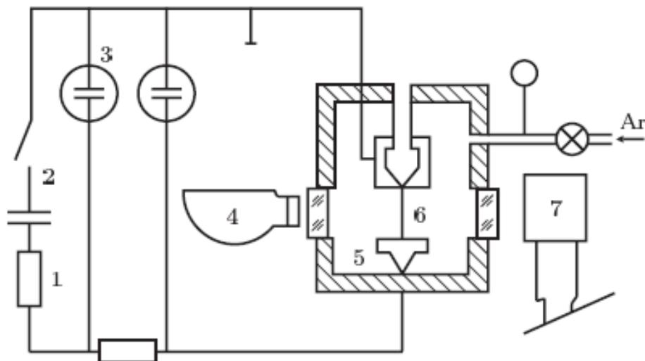
Figure 3. Schematic diagram of the experimental setup for exploding wire method. 1 - ballast resistor; 2 - capacitor bank; 3 - oscillograph; 4 - high-speed photorecorder; 5 - high-pressure chamber; 6 - heated wire; 7 - spectrograph.
