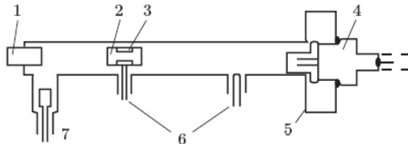
Figure 4. Schematic diagram of high pressure discharge tube. 1 - quartz window; 2 - auxiliary electrode; 3 - steel ring; 4 - pressure sensor; 5 - cathode; 6 - tungsten probes; 7 - anode.
