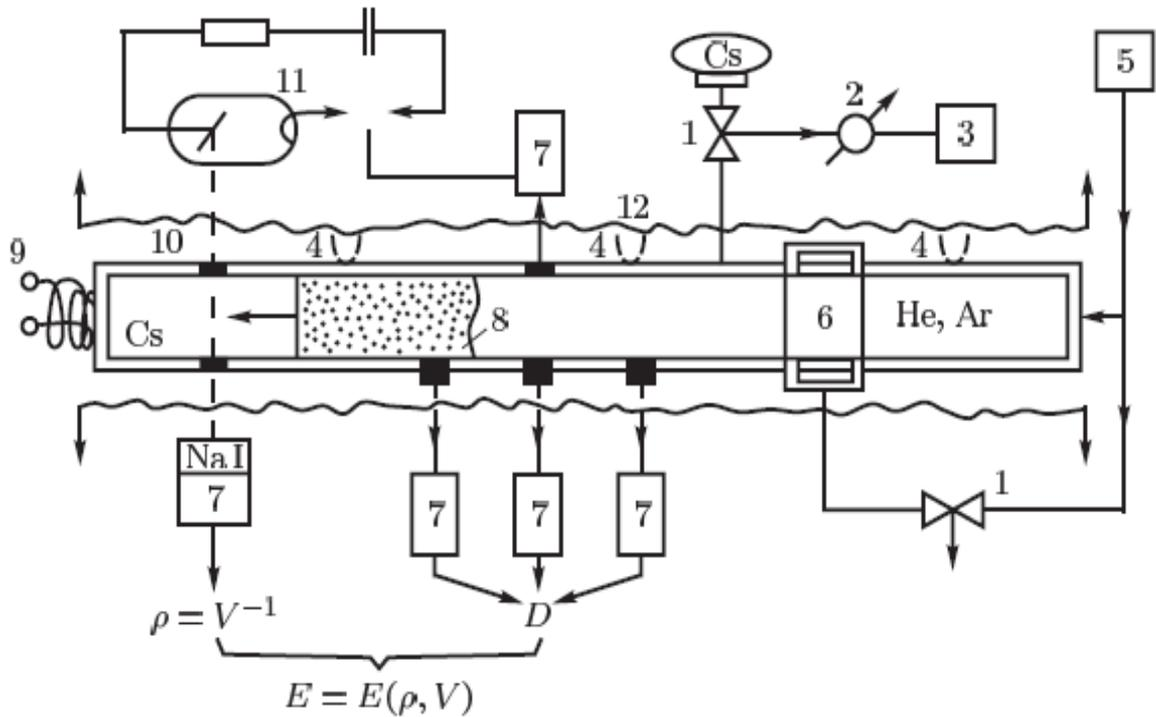
Figure 6. The schematic diagram of a heated cesium shock tube. 1 - air-operated valves; 2 - system for measuring the initial cesium pressure; 3 - liquid cesium vessel; 4 - thermocouples; 5 - propelling gas; 6 - diaphragm unit; 7 - photomultipliers; 8 - shock-compressed plasma; 9 - electrical conductivity measuring coil; 10 - beryllium windows; 11 - X-ray tube; 12 - electric heater.
